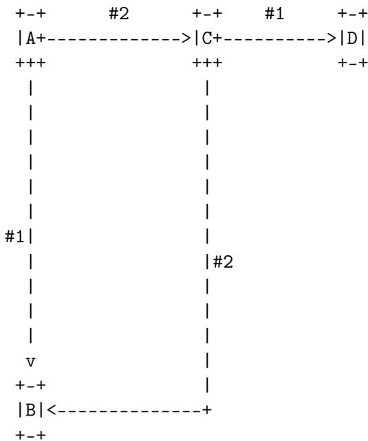
Router A has two out-edges, its #1 out edge is connected to Router B and its #2 out edge is connected to Router C.
