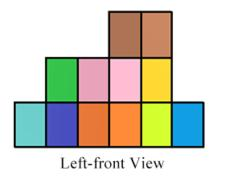
The left-front view can also be regarded as a projection onto a plane, while the plane is at an angle of 45° to the left view's plane and the front view's plane. The following picture shows how it projects in a top view.
