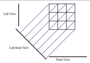
Therefore, if we regard the top view as a grid with n rows and m columns, the left-front view should have n + m columns.
